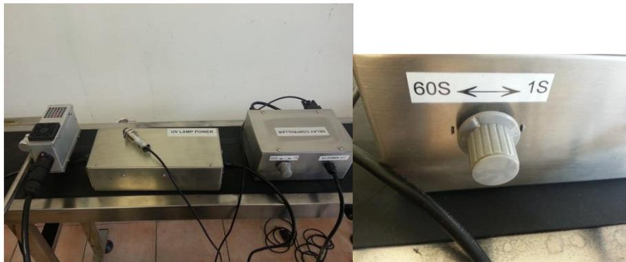
1 uv curing lamp, 2 power transformer ,3 lamp time control automatic on /off timed controlled UV
